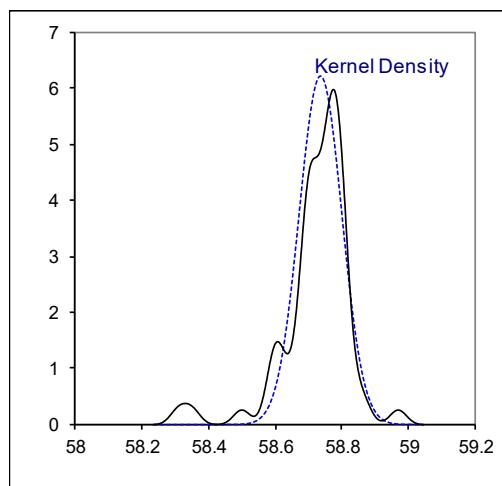
Determination of Aromatics by FIA (without oxygenates correction) on sample #21015; results in %V/V
